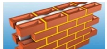
Regular brick pattern of a cavity wall
