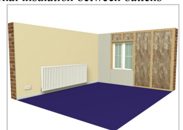
Internal insulation between battens
