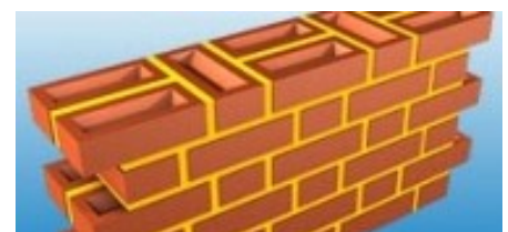
Alternating pattern of a solid wall
